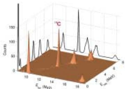
AMS spectrum measured for  $^{14}\text{C}$  from a modern charcoal sample. In the sample the  $^{14}\text{C}$  concentration is  $10^{-10}$  atomic percent.
